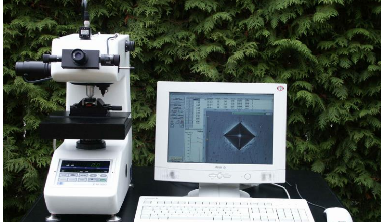
Full automatic ecoHARD® Case Depth Measurement System from AHOTEC® e.K., 2001
