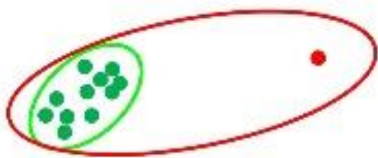
Figure 9 – Tolerance field included a NOK part
